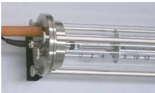
Energy loss measurement of \alpha -particles in air
