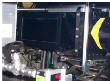
Plastic scintillator ( TOF ) @ S4
