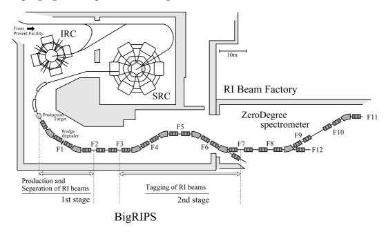
Figure 1: Overview of the RIBF facility. The radioactive ion beams are produced and separated with the BigRIPS fragment separator and transported to the focus F11, the location of the E(U)RICA spectrometer.
