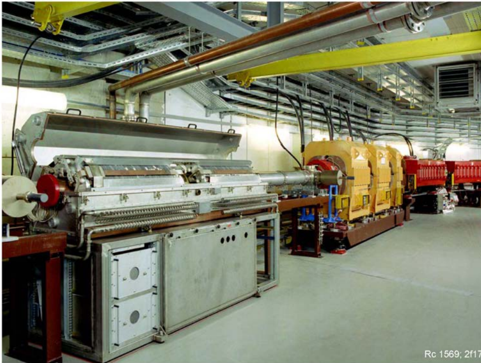
SIS-18 accelerating cavity
