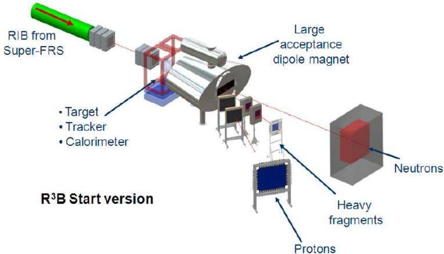
Excitation energy E\* from kinematically complete measurement of all outgoing particles
