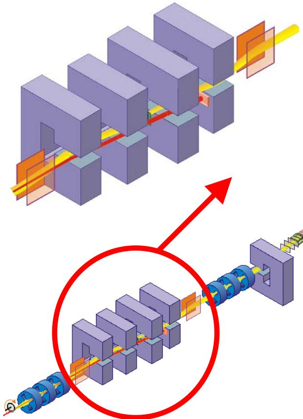
electric deflectors:  $\pm 330$  kV    dipole magnets: 0.7 T max
