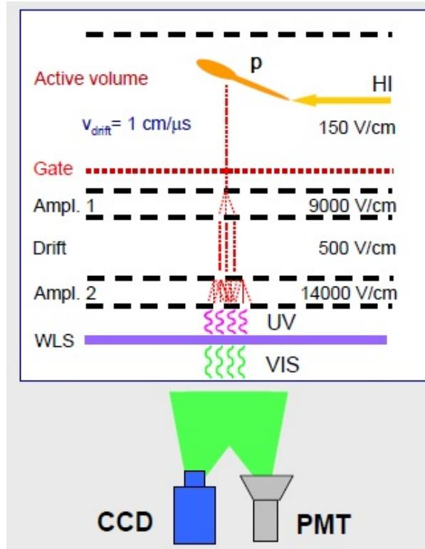
Gaseous ionization detector (TEA = Triethylamine  $\text{N}(\text{C}_2\text{H}_5)_3$ ) developed to measure the angular and energy correlations between the protons emitted in 2p decay of  $^{45}\text{Fe}$ .
