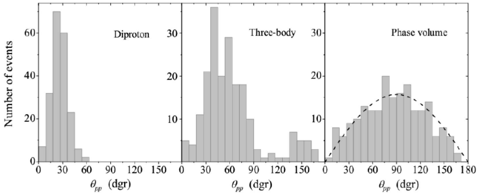
Monte Carlo simulation (200 events) of the [opening angles](#) between both protons for the  $^{45}\text{Fe}$  decay
